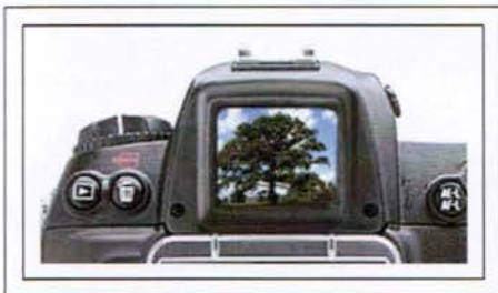
Fig. 5: Most of the electronic viewfinders (EVFs) in digital still cameras are very small LCDs, which make substantial demands on the backlights that illuminate them.
