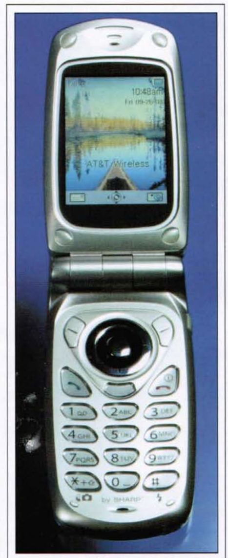
Fig. 4: A camera-equipped mobile telephone with a high-resolution color display, such as the Sharp XG28 with a CG-Silicon display, is a prime example of a convergent device.
