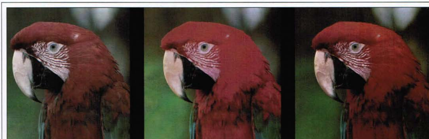
Fig. 3: The photograph on the left shows a typical mobile-display image without color processing; the image looks rather pale. By simple color processing, the photograph in the center shows improved colorfulness, but with visible clipping artifacts. Advanced color-gamut mapping shown on the photograph on the right preserves the colorfulness while eliminating clipping artifacts.
