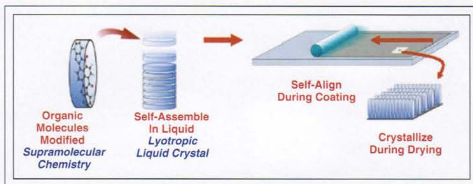
Fig. 1: The Cascade Crystallization process forming thin crystalline films consists of a chemical-modification step and four steps of ordering that form the crystal film.
