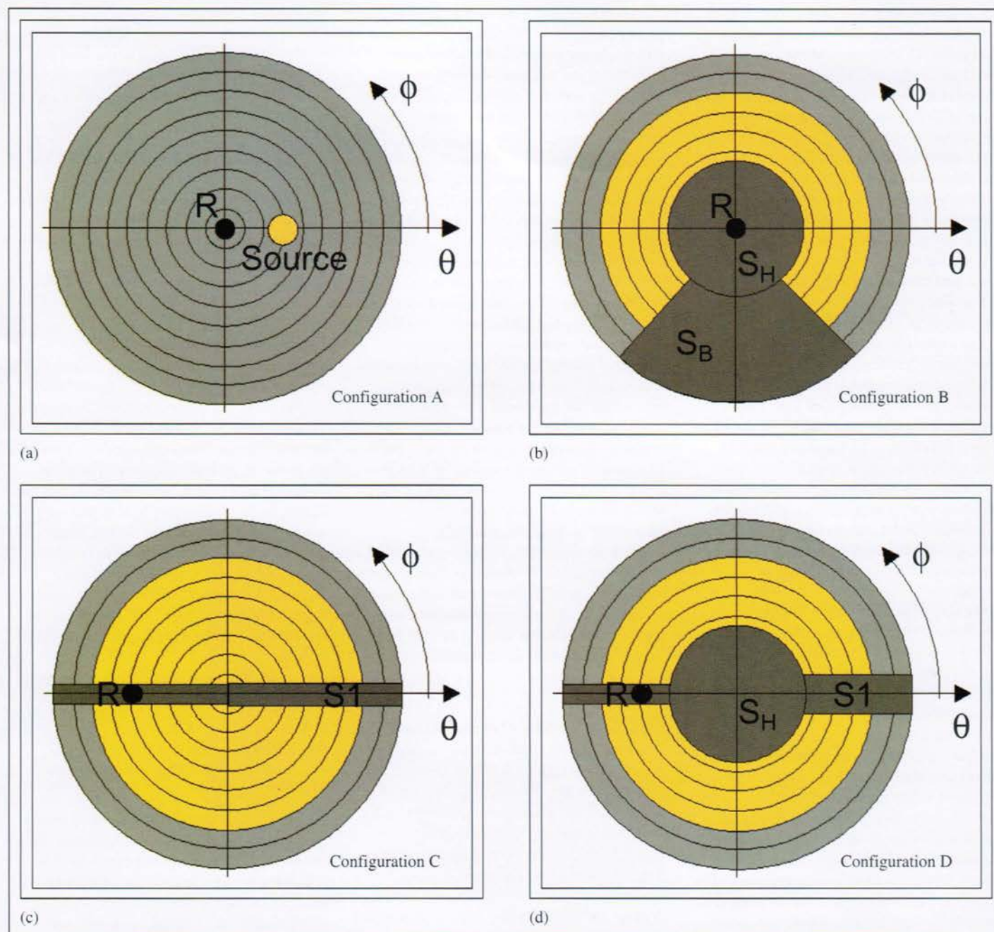
Fig. 2: Four basic illumination geometries are shown in polar representations: (a) “directional” illumination at 30^\circ with a fixed receiver (R); (b) multi-directional illumination shaded by the head ( S_H ) and shoulder and trunk ( S_B ) of an observer and fixed receiver (R); (c) multi-directional illumination with shade and gloss trap ( S_I ); and (d) multi-directional illumination with head shade ( S_H ) and gloss trap ( S_I ), both with variable receiver inclination for scanning of the viewing cone.
