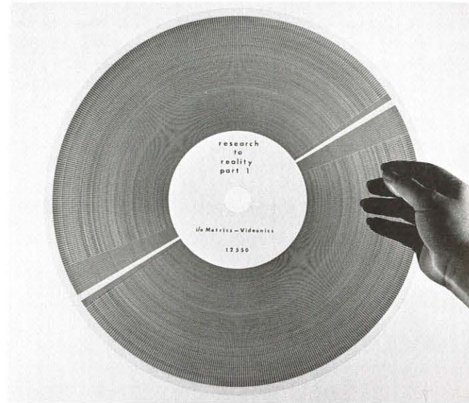
Figure 3. Appearance of the video film disc. This particular disc has a playing time in excess of 20 minutes at the full NTSC video framing rate.
