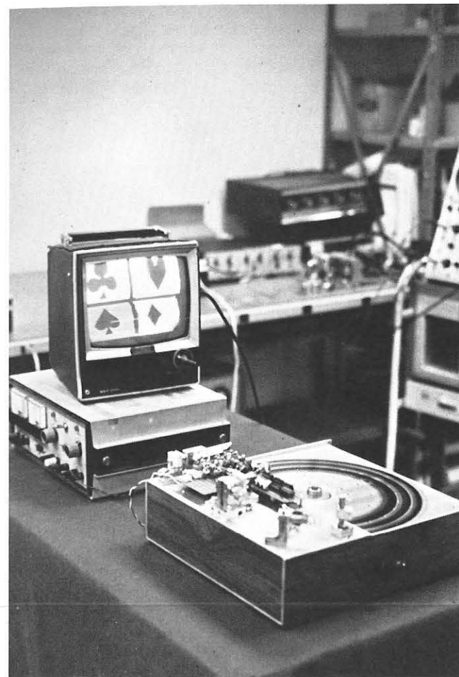
Figure 8. The video frame presented on the monitor is constructed from four different data tracks on the disc. There is one read-head (photodiode) per track, with an electronic switch between tracks effected twice per line and twice per field.
