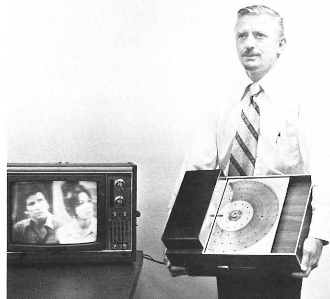
Figure 6. The video signal displayed is generated directly by the hand-held video player, demonstrating operation under environmental stress.
