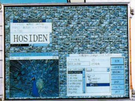
TFT active matrix LCD module HLD1201 31 cm (12.1 inch) 800(X3)×600 dots (262×10 3 colors)
