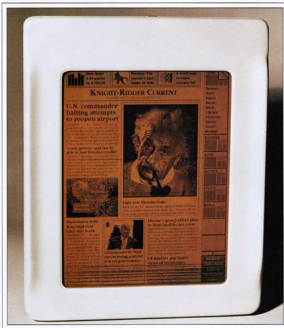
Fig. 4: This full-page-size 1152 × 896-pixel bistable reflective cholesteric display has a contrast ratio of 20:1 and wide viewing angles.
