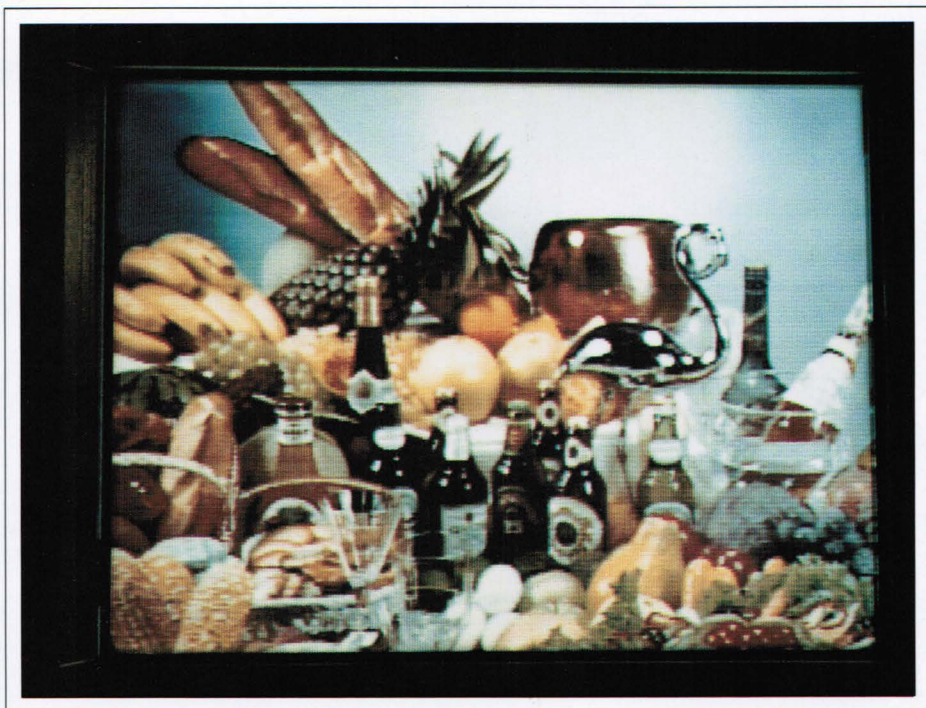
Fig. 5: The wide viewing angle and lack of color inversion in this anti-ferroelectric LCD, which Nippondenso demonstrated at SID '95, resulted in a very attractive display.
