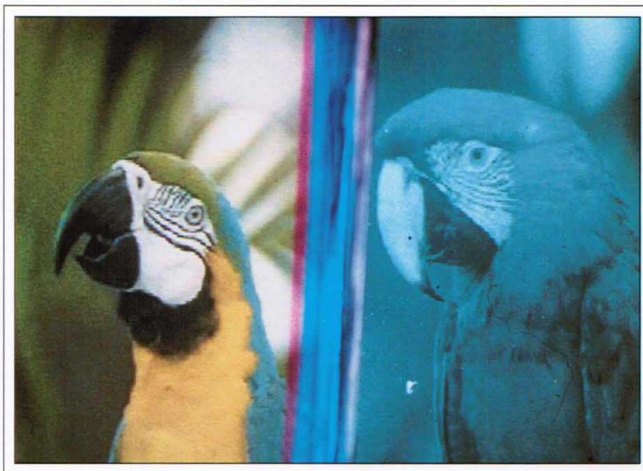
Fig. 2: A switchable color filter based on FLC technology is placed so that it covers only the left half of a 1.5-in. monochrome CRT showing a VGA image (unaltered Extachrome™ transparency).
