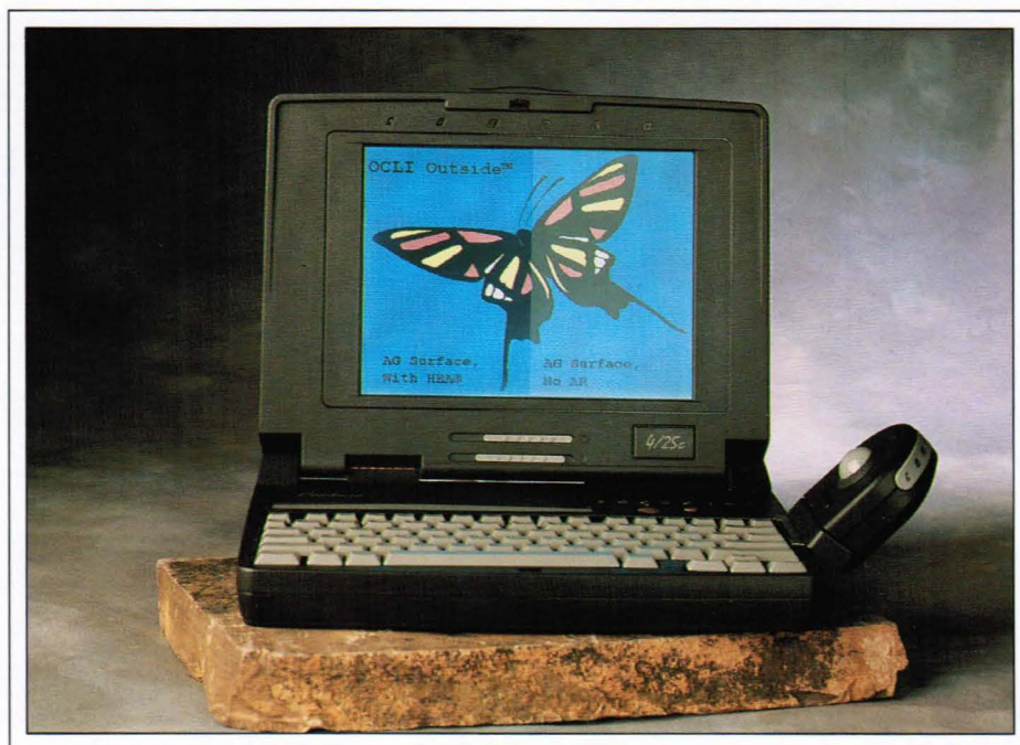
Fig. 1: As part of a test, an MLAR-coated polyester film was laminated to the AG surface of the polarizer on the left half of this commercially available color STN display.
