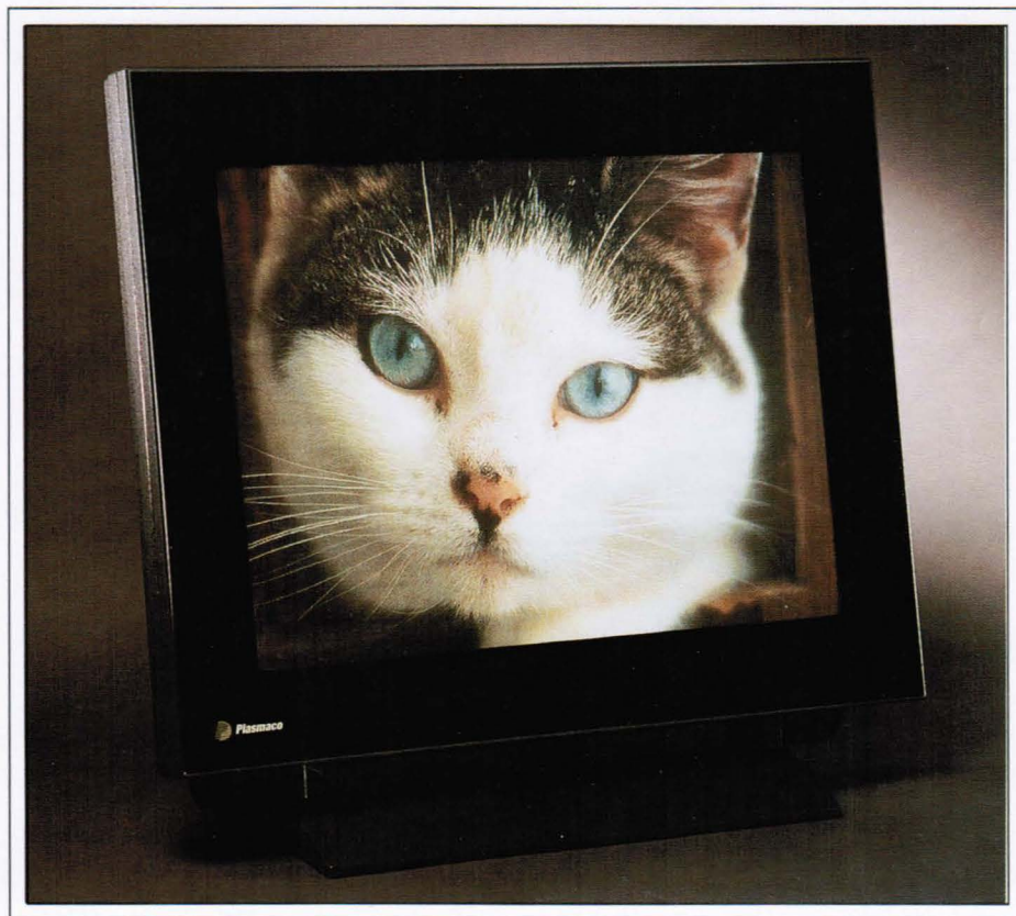
Fig. 1: Plasmaco surprised the cognoscenti by introducing its first color ac plasma-display prototype at SID '94 after a remarkably short 5-month development effort. Shown on the 21-in. 640 \times 480-pixel display is a full-color image produced by the panel's 24-bit drive electronics.
