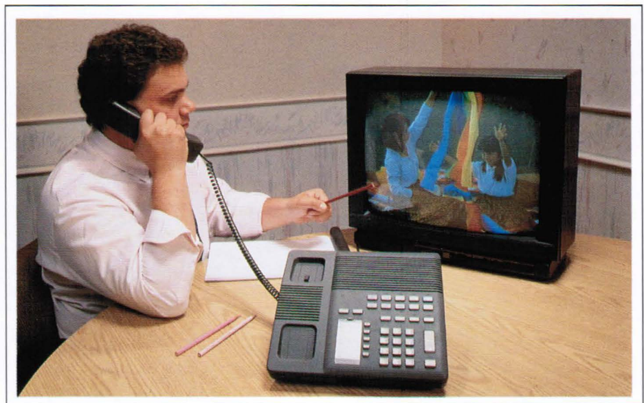
Fig. 1: The Picasso Image Telephone allows users to send full-color NTSC-quality still images and simultaneously talk over the same dial-up analog phone line.
