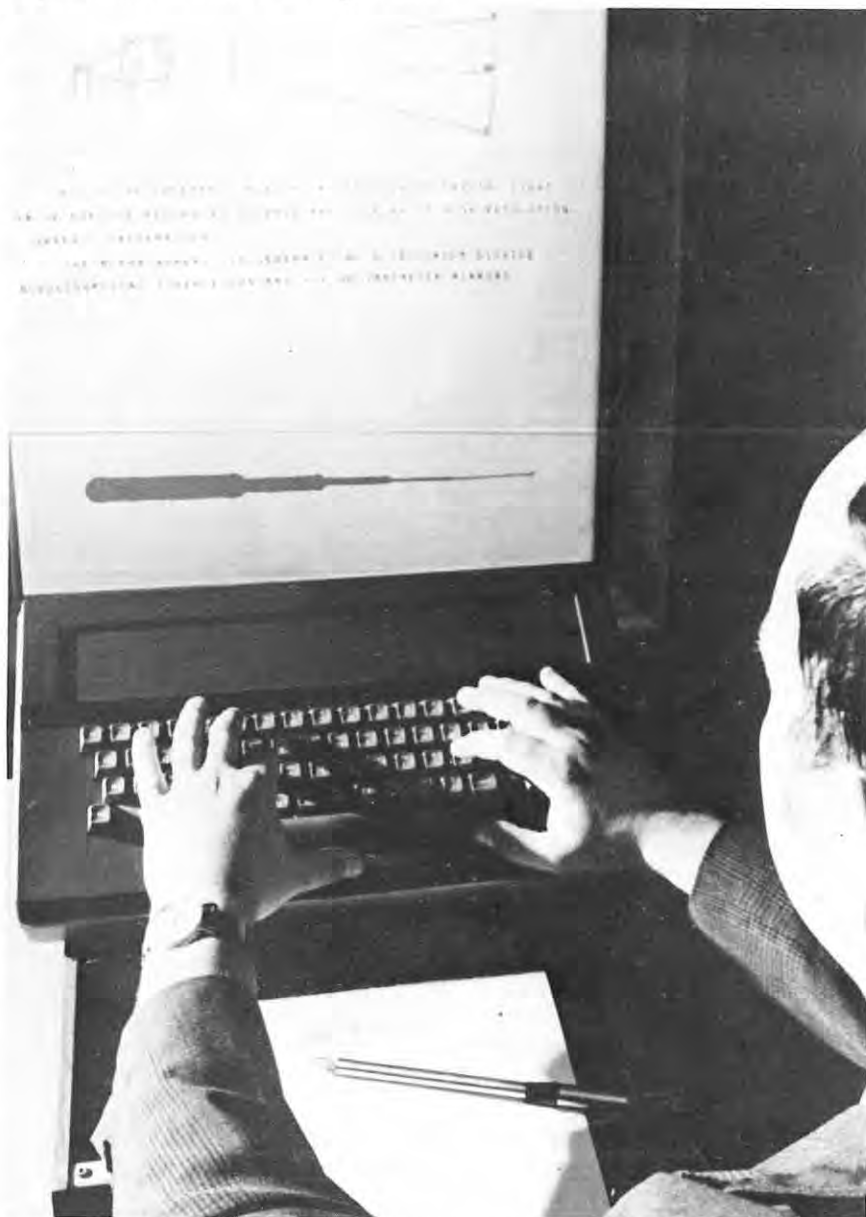
Demonstrating how words and drawings can be projected through a glass filled with a liquid crystal chemical compound.
