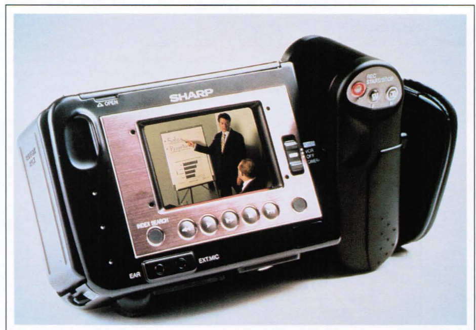
Fig. 5: The new Viewcam™ VL-E30UP by Sharp Corp. uses a 3-in.-diagonal color a-Si TFT-AMLCD for its innovative viewfinder. This new application of LCDs, which required increased viewing angle and decreased reflectivity, has had a major impact on camcorders.
