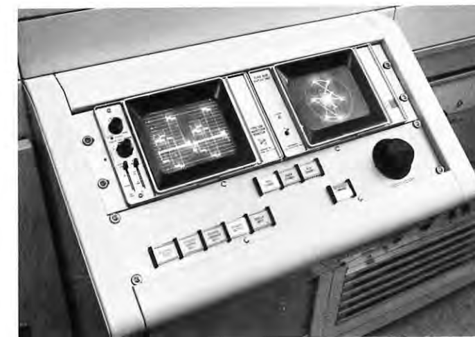
Figure 5: Selection panel for test signals allows system performance to be checked prior to recording.
