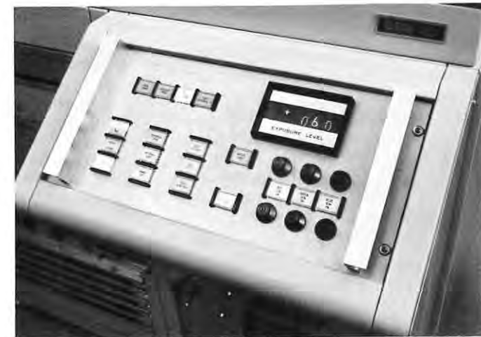
Figure 4: Controls for selection of results of film transfer are grouped to aid operator in correct sequence of operations.
