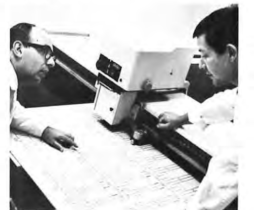
A production mask for a machine part—drawn on film by a light beam automatically controlled by computer commands—is checked by draftsmen at the IBM Systems Development Laboratory in San Jose, California. The path of the beam is directed by an experimental computer program for high-precision graphics.
