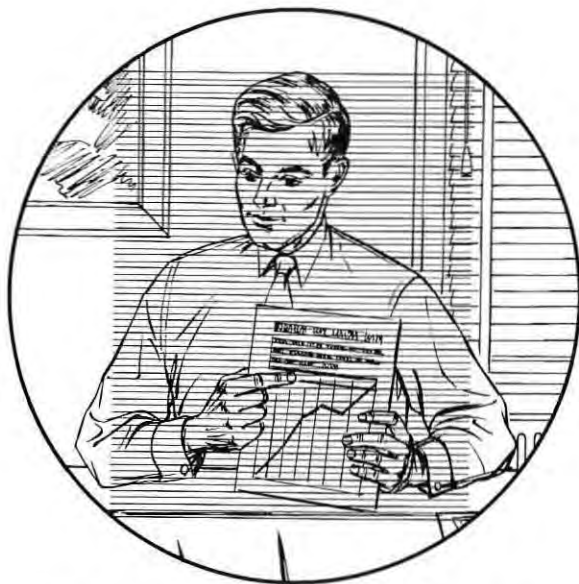
Formation of the conventional interlaced raster. Circular boundary of the illustration encloses the image the camera lens forms on the target of the tube. The rectangular area of horizontal lines—the raster—defines the transmitted image. Each field of the raster is scanned in a sixtieth of a second, the two scanings comprising a frame. Frame rate of 30 per second assures normal animation in the displayed picture. Field rate of 60 per second precludes broad area flicker.
