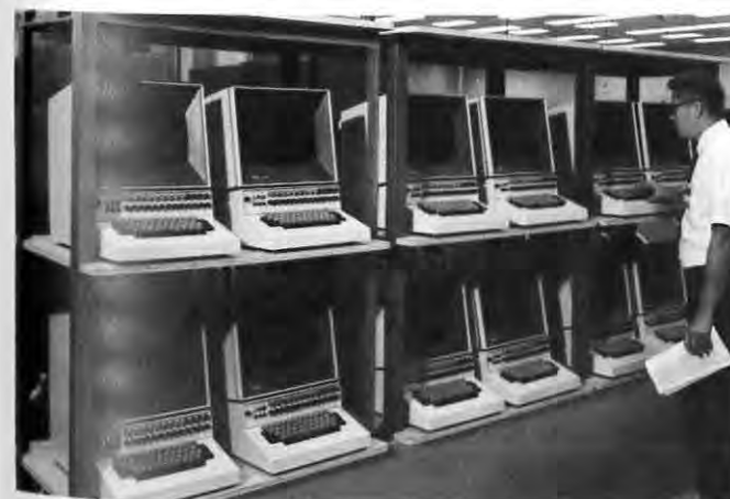
The 24-channel keyboard data entry simulator, housed in three frames. The single-shot timing capacitors are externally attached to provide flexibility. The record-length counters are located across the top of the frames.
