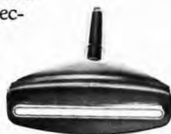
Fig. 2. SC-3154 high-resolution electrostatic printing tube with useful screen area of 0.16" x 8.6".
