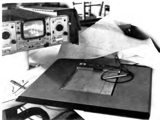
FIGURE 1: User sketches with pen-like stylus on "Grafacon" tablet. The CRT monitor displays a record of the input data allowing careful position checking and error determination.
