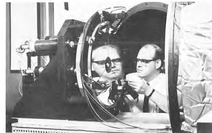
Perkin-Elmer scientist Hugh J. Robertson makes final adjustments on segmented mirror for Active Optics program.
