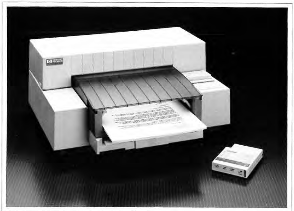
Fig. 1: At its Boston Fall Print Quality Conference during the last week of October, DATEK gave its Printer-of-the-Year Award to the Hewlett-Packard DeskJet—the plain-paper drop-on-demand ink-jet printer that produces laser-quality output.
