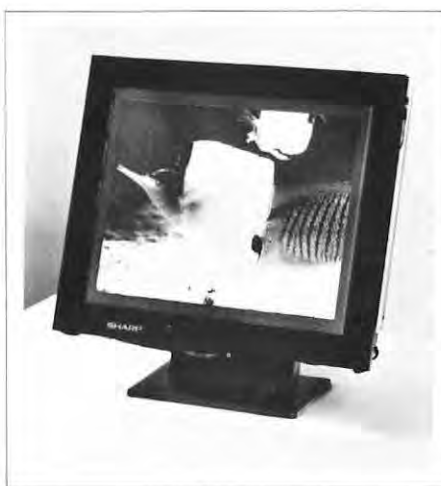
Fig. 1: In August, Sharp demonstrated a 14-in. full-color matrix-addressed liquid-crystal display—the largest yet. Sharp is promising evaluation units during the first half of 1989.
