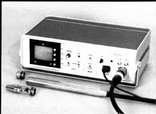
ISTC's underwater camera is a complete TV inspection system specifically for nuclear reactor use.
