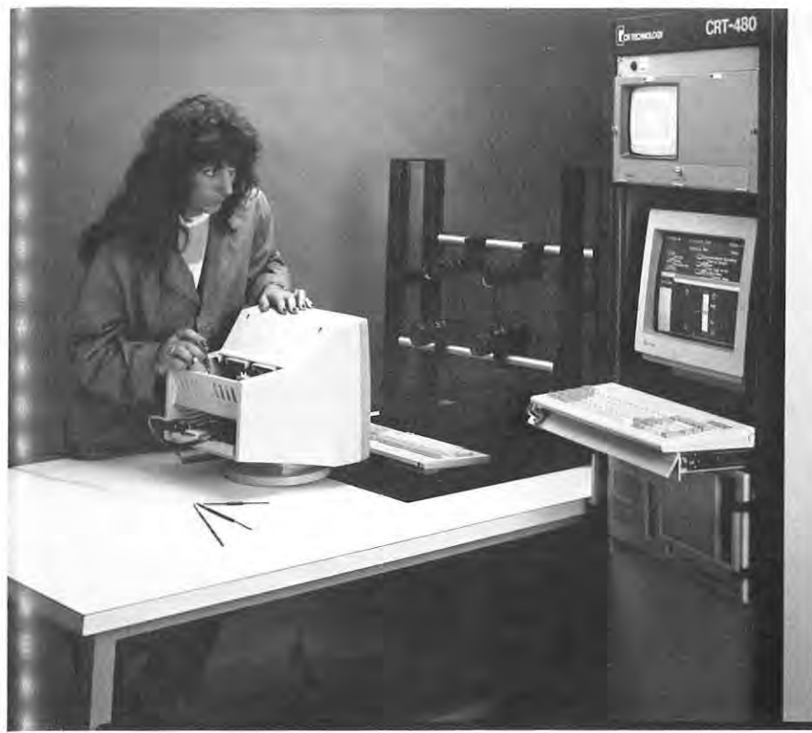
Fig. 1: Semiautomated CRT adjustment uses machine vision and a graphic interface to enhance the operator's performance. In this adjustment for image height, the screen of the CRT under test is imaged by CCD cameras and sent to an image processor and an Intel 80386-based microcomputer. When the operator has set the height to within the programmed tolerance, the test system provides visual and audio confirmations. In a manufacturing environment, such a test system would be placed on the production line.
