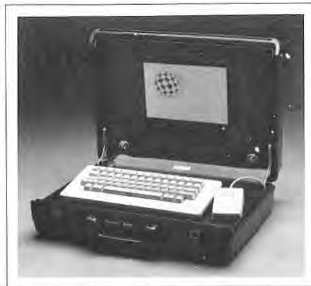
Fig. 1: An experimental briefcase computer with a plasma display using low-cost drive circuitry. The computer functions as an Apple Macintosh.
