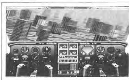
Fig. 3: DVI's fast video display processors can recalculate the warps for an entire screen several times a second, permitting highly realistic flight simulators.
