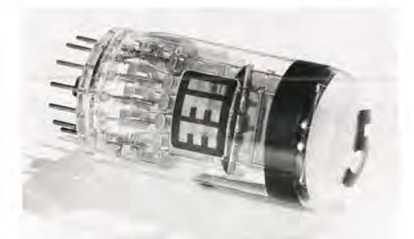
One of 10 flood guns operating on 10 V swing.
