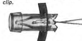
Neon lamp in base with short cylindrical filter (available in colors) and spring retaining clip.
