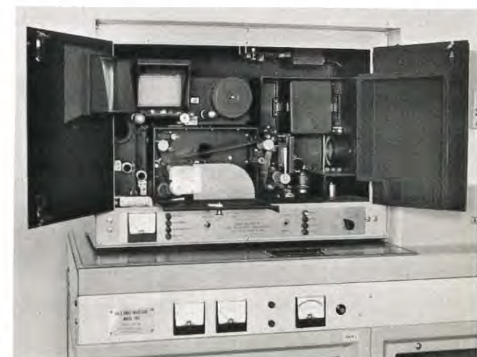
FIGURE 5: Upper section of Nimbus processor showing Bimat supply container (center), laminating rollers (to left of container), negative film viewer (top left), and camera section (right).
