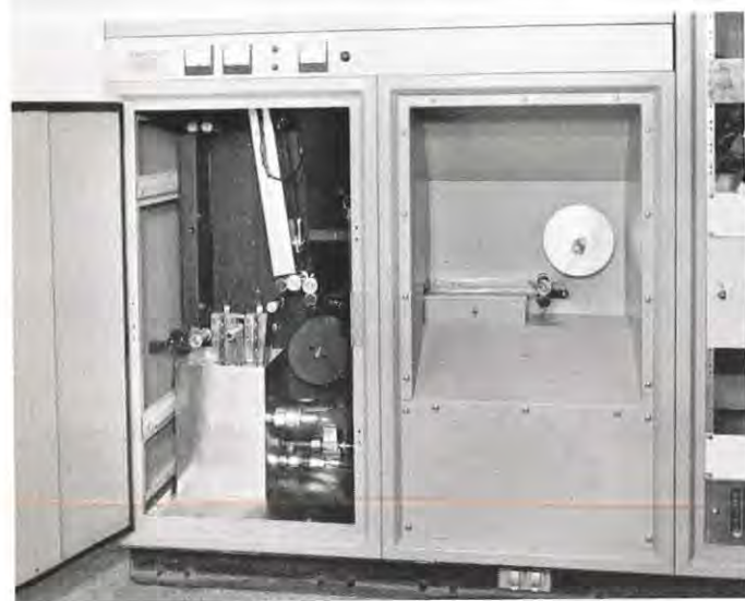
FIGURE 6: Lower section of Nimbus processor showing processing tunnel, wash tank (lower left), cover sheet supply spool (black), and positive image take-up (right).
