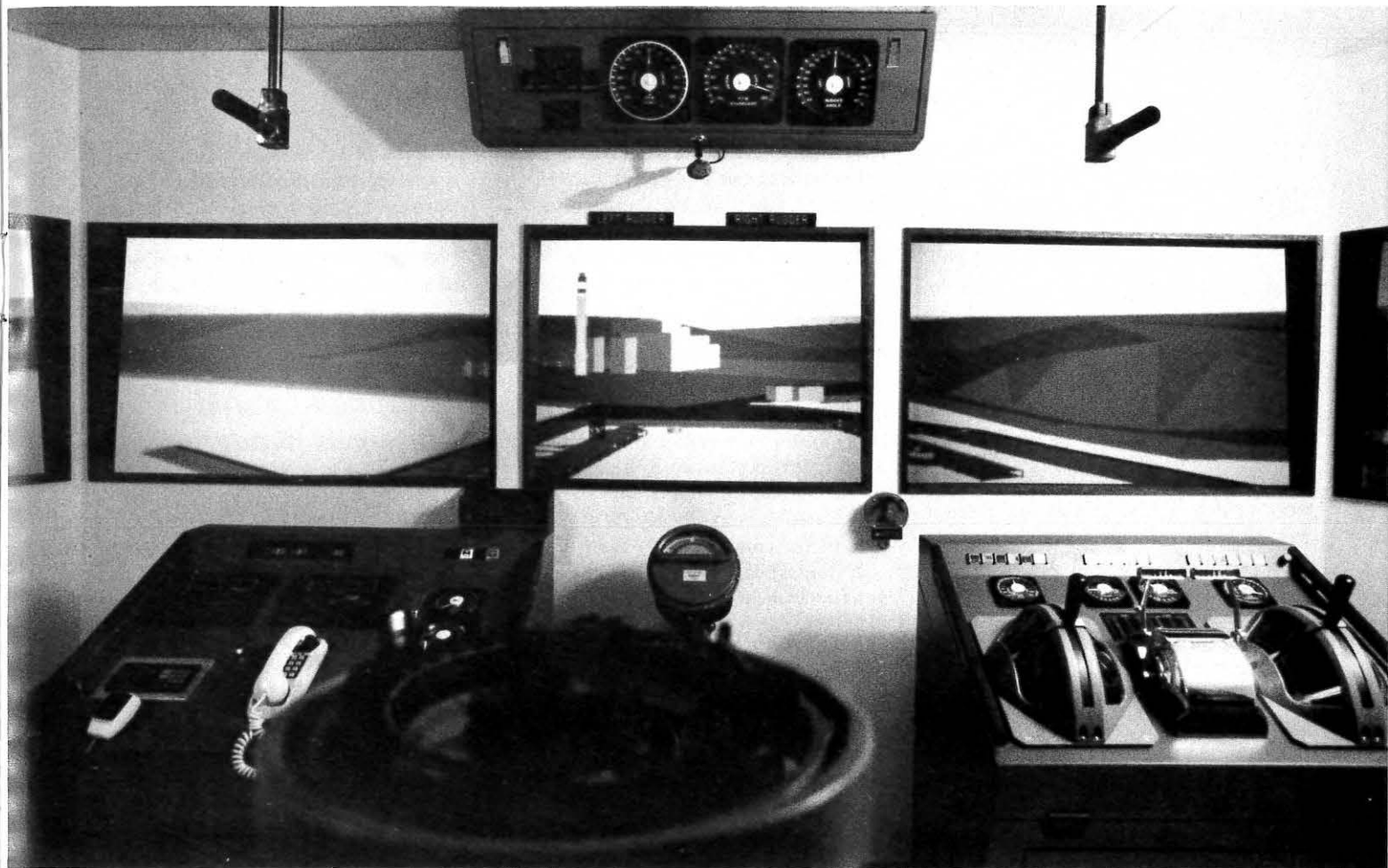
Fig. 1: Part of the view from the "bridge" of a shiphandling simulator. The full display spans seven "windows" with a 182° horizontal field of view. The display changes in response to inputs from the bridge controls, takes into account wind, currents, tides, and the programmed characteristics of the ship being simulated.
