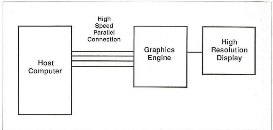
Fig. 2: Typical configuration of a high-performance graphics system.
