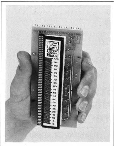
both trend and four-place digital accuracy. The module is  $2.1 \times 5.8$  in., with a  $5 \times 0.5$  in. LCD. The cost is \$229.90 ea. at 100 pieces.
