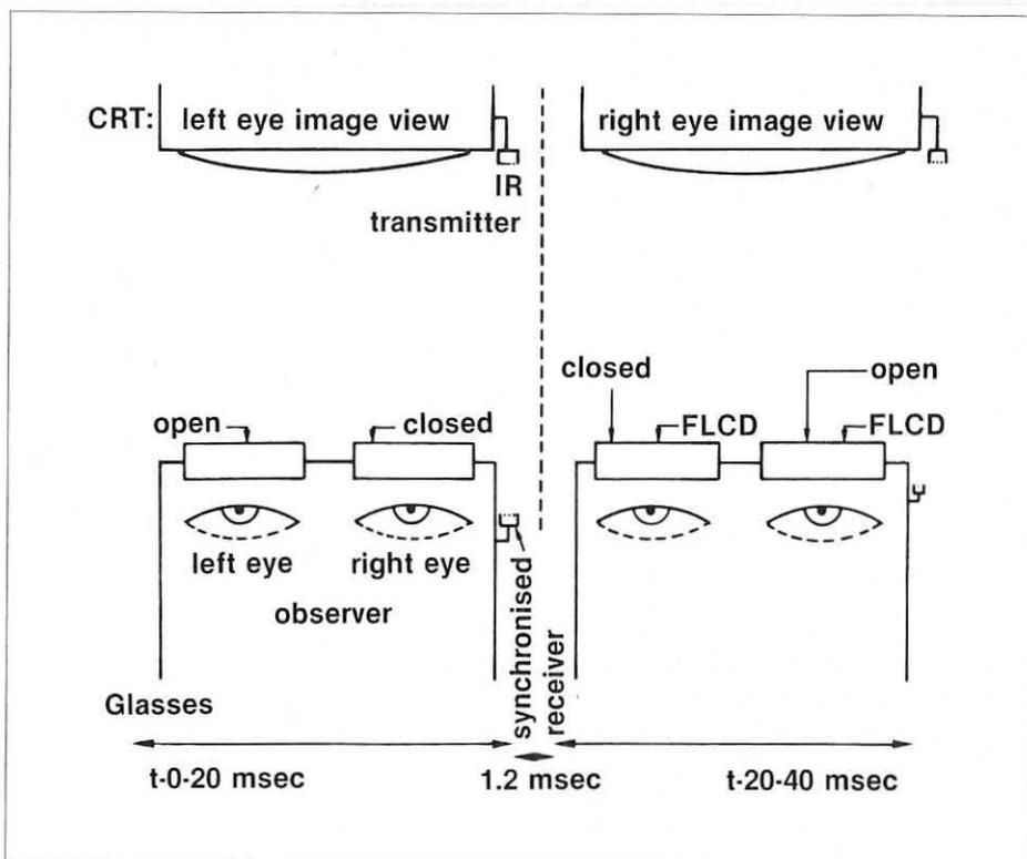
Fig. 1: Field-sequential stereoscopy.
