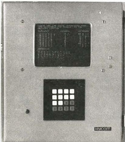
NETWORK MONITORS display computer data at remote locations. The host computer can service up to 64 monitors (RS-232/RS-244). A local keypad requests data and selects desired page for display. Local memory holds three pages. TFEL page matrix can be 320 × 240, 512 × 256, or 640 × 200. Self-powered; NEMA enclosure; output for serial printer.
