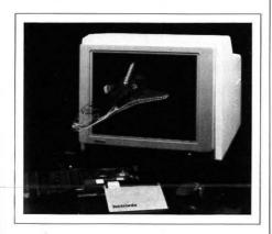
The Tektronix stereo graphics system uses a time-multiplexed stereogram technique involving the construction of a video frame containing separate sequential video fields for the left- and right-eye images. The liquid-crystal modulator encodes these images with left and right circular polarization for both eye images. The complete SGS 430 system costs \$9800.
