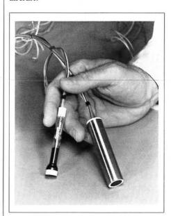
The IM70P53MFO tube provides an 0.0008-in. line width across a 0.4-in.diameter useful area and a 500-fL area brightness through the integral fiber optics faceplate. A low inductance coil is precision aligned within a mu-metal shield. Maximum weight, excluding lead,
