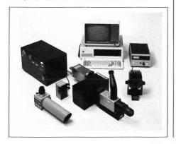
precise, accurate, and repeatable measurements, the C-11ASR was used to create military specification MIL-L-85762. The C-11ASR ensures that cockpit lighting and instrumentation will not interfere with the operation of night vision goggles, thus increasing the safety of pilots and crew. In addition, the C-11ASR can quickly and easily be reconfigured to do spatial analyses, and even secure lighting measurements.
