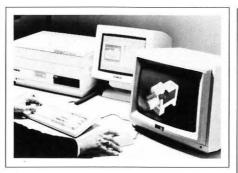
reduction time for slides and other graphical material. The GDW's TVresolution frame stores provide 8 bits/pixel, giving high-quality 256-level gray scale output, or a true-color 24-bit output when three cards are fitted, at a display resolution of  $768 \times 575$  pixels.
