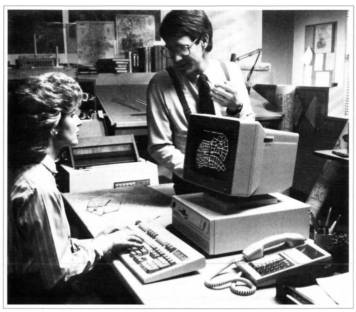
Fig. 1: IBM's 80286-based desktop model 50 and the new Personal System/2 monochrome display model 8053 being used to plot a subdivision. In the background, and IBM Quietwriter (R) III printer is ready to produce high-quality graphics.
