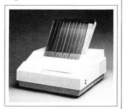
The printer uses sequential overprinting and color mixture techniques to produce a high-resolution graphics output in seven basic colors and allows for over 200,000
