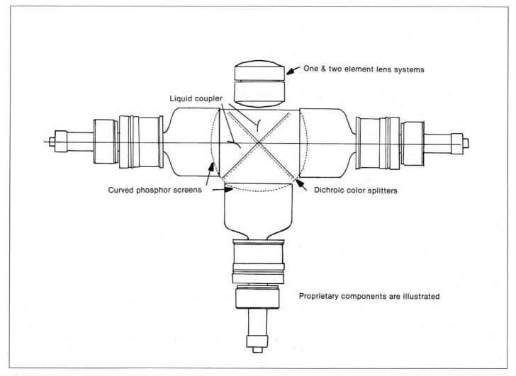
Fig. 4: Triuniplex CRT projection system.
