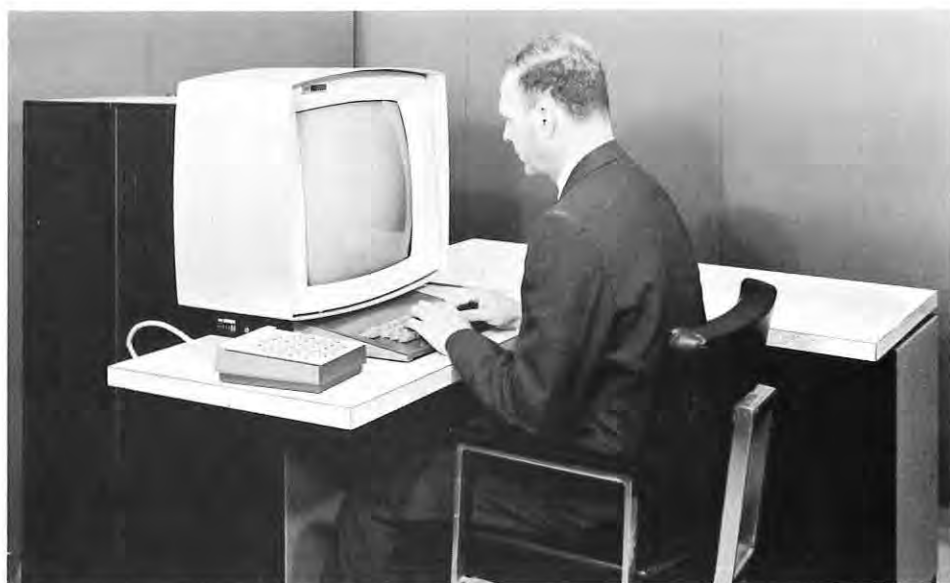
FIGURE 4: The IBM display systems are direct-view CRT display consoles designed for single- or multiple-console installations. Multiple units can be separated from their control units by up to 2000 ft. of cable. Detection, tracking and sketching can be performed with a light pen.
