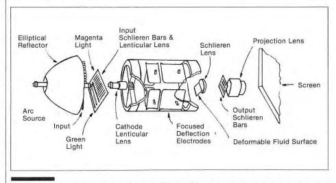
Fig. 3: For somewhat smaller displays, General Electric's Talaria light-valve projector offers certain advantages over the older design of the Eidophor.
