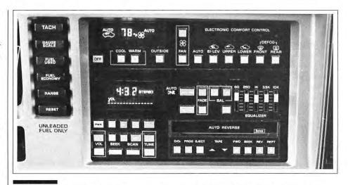
Fig. 1: A conventional top-of-the-line automobile dashboard, above, uses pushbuttons that are dedicated to controlling a single function. More features mean more crowding on the dash panel. Fig. 2: The touch interactive graphic control panel, below, uses touch-panel-over-CRT to provide simplified, reconfigurable switching. Summary "page" of the display is shown, one of 39 available to the driver; additional diagnostic pages can be accessed by a service technician.
