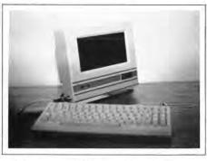
A light-emitting flat-panel terminal from Emerald Computers, Inc. combines previously unutilized flat-panel benefits and conventional system access technology. The device has been designed to provide multiterminal users with a light, durable, compact alternative to conventional CRT terminals, without the disadvantages of electromagnetic distortion, mechanical vulnerability, eye strain, and ambient radiation.
