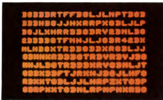
Figure 6. Photo—Alphanumeric Pattern of Entertainment 14V CRT, 3000 Characters/Frame.
