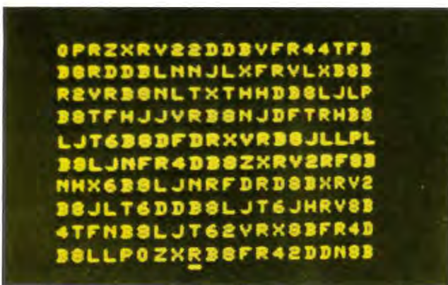
Figure 7. Alphanumeric Pattern of Electrostatically Focused High Resolution, 2-Color CRT, 3000 Characters/Frame.
