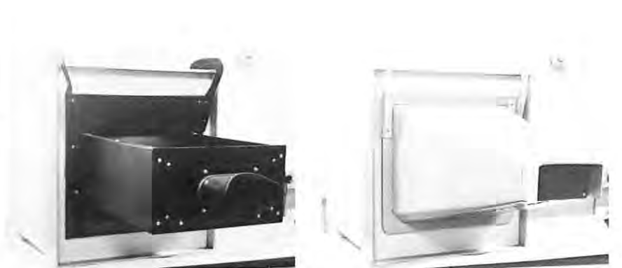
Figure 4. Photographs of (a) a mirror stereoscopic attachment and (b) a prism stereoscopic attachment.
