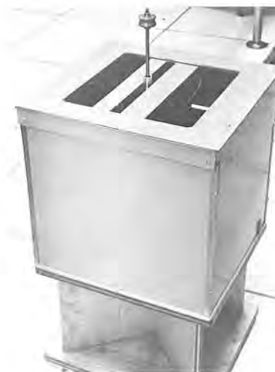
Figure 7. Photographs of a three-dimensional cartesian input device both (a) with and (b) without external covers.
