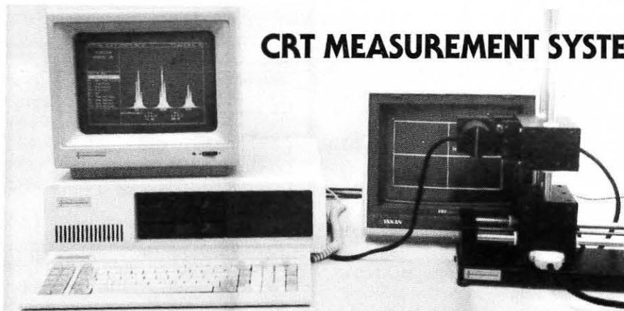
Automatic, direct convergence measurements on CRTs are now possible with the SUPERSPOT 100. Line width, MTF and many more CRT measurements are made accurately and in real time with data logging, profile plotting, as well as real time adjustment of convergence and focus.
