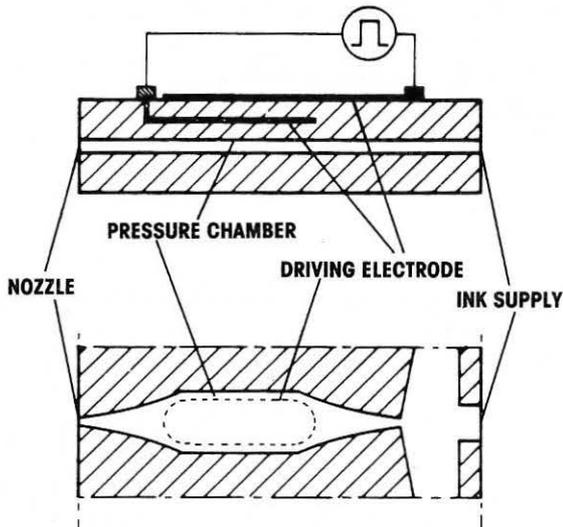
Driving electrode for the piezoelectric actuator is oblong with two semicircular sides, whose short length and area are 2.75 mm and 19.7 mm<sup>2</sup>, respectively.
