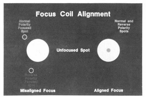
trajectory—causing them to converge towards the phosphor screen. A single-gap, thin lens with both static and dynamic windings produces the focusing fields.
