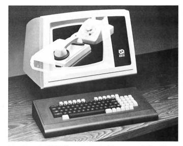
Lear Siegler's ADM 32 smart terminal is now available with an integral modem capable of operating at either 1200 or 300 baud. The new modem eliminates the need for a telephone and an acoustic coupler by enabling the telephone line to be plugged directly into the terminal.
