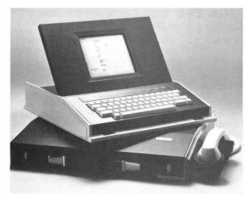
Kylex portable display terminal fits into an attache case because of its compact LCD.
