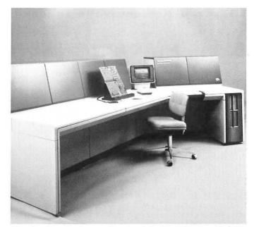
Marathon functional test stations are derived from the Capable 4900 line of real-time functional testers. These stations offer test pattern speeds of up to 16 MHz data rate, 4 MHz test cycle rate, and up to 1024 pins with interchangable high-speed programmable interfaces.
