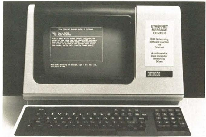
One of the Comdex Ethernet message stations consists of a DEC VT103 terminal with a plug-in LSI-11 processor. It is also equipped with 3Com's new Q-bus Ethernet controller and UNET software running with the Xenix operating system.
