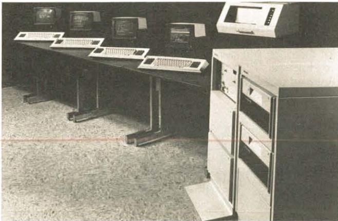
FailSafe System Introduced by Dosc, Inc. The FailSafe on-line computer system, said to incorporate significant advances in automated software development and fail-safe hardware architecture, has recently been introduced by DOSC, Inc., of Albertson, N.Y. Shown are system workstations (left), a high-speed printer, and fully-redundant data base discs and data base manager computers (right).
