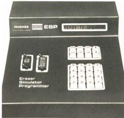
New Eraser/Simulator/Programmer, from Hughes Aircraft Company's solid state products division, supports the company's currently available EEPROMs, plus additional non-volatile memories planned by Hughes. The microprocessor-controlled smart programmer, designated H3000 ESP, can erase, program, read, copy simulate, modify, and compare a variety of PROMs, without requiring personality boards, hardware changes, or switch settings for different memory and parameter selections.
