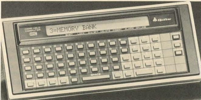
Hand-held computer from Quasar Company, Franklin Park, IL, features a 6502 microprocessor, and is programmable in Microsoft™ Basic and SNAP, a FORTH-like language. Optional peripherals connect the computer to large mainframes and databases over telephone lines, and to a conventional television receiver for local display. A thermal printer, RS 232C interface, and extra memory are also available.
