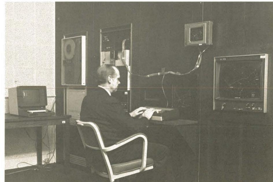
displays which can currently be demonstrated include a 512 x 512/60 lpi plasma matrix, a 256 x 512/60 lpi plasma matrix, a 240 x 320/68 lpi electroluminescent (EL), a high resolution shadow-mask color CRT, a standard (home TV) shadow-mask color CRT, and a 3-color beam penetration stroke-written CRT. Samples of 7-segment EL, large screen TV, and EL TV can also be demonstrated. Lighting conditions can be controlled to observe the effects of ambient lighting conditions varying from dark-
