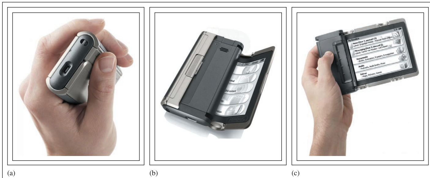
Fig. 1: (a) When the display is closed, the RADIUS measures 115 mm long, 21 mm thick, and 57 mm wide. (b) The display is only about 100 \mu\text{m} thick, about 10 times thinner than glass displays of similar size and about 5 times thinner than current plastic displays. This allows it to bend easily as well as to roll and unroll frequently without any degradation to image quality. (c) When fully extended, the display measures about 5 in. on the diagonal and extends the device to a width of 160 mm.
