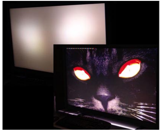
FIGURE 1 — Illustration of local dimming. The backlight (rear image) is at full brightness at the position of the cat's eyes and is dimmed at the darker parts of the image. The panel (front image) is simultaneously compensated for the backlight modulation such that the scene is properly depicted.
