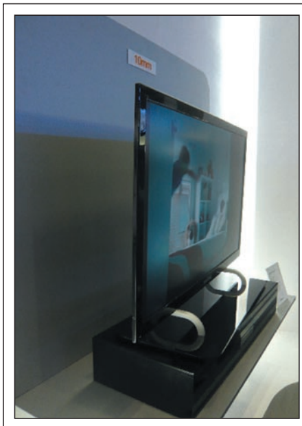
Fig. 1: The 10-mm-thick LCD-TV module.
