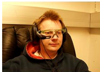
FIGURE 2 — The participants viewed a small NED placed either approximately 5° above or approximately 15° below the horizon line of sight. The ViewSonic display's middle point was approximately 5° below the horizon line.
