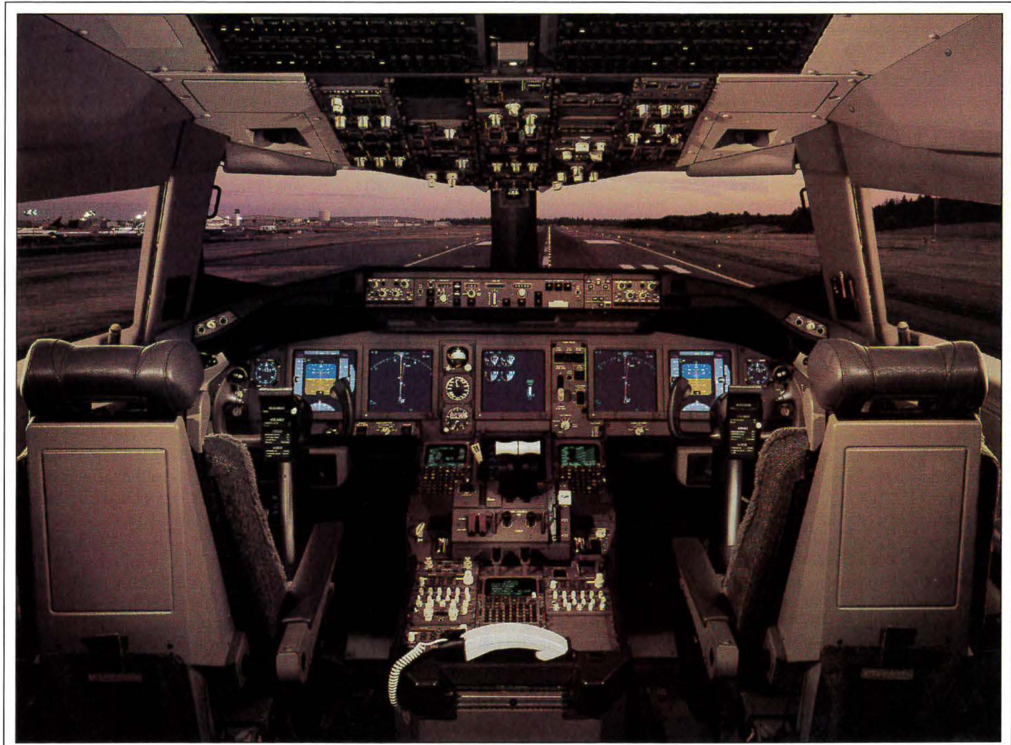
Fig. 1: This state-of-the-art "glass cockpit" is standard issue in Boeing's new 767-400ER. Display layout and format are common in the Boeing 777. The displays and system integration for the 767-400ER are by Rockwell Collins.
