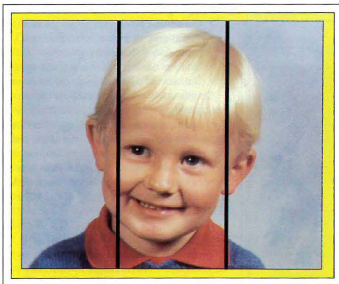
Fig. 3: This simulated image suggests the appearance of a tiled display with visible seams in a 1 × 3 array.
