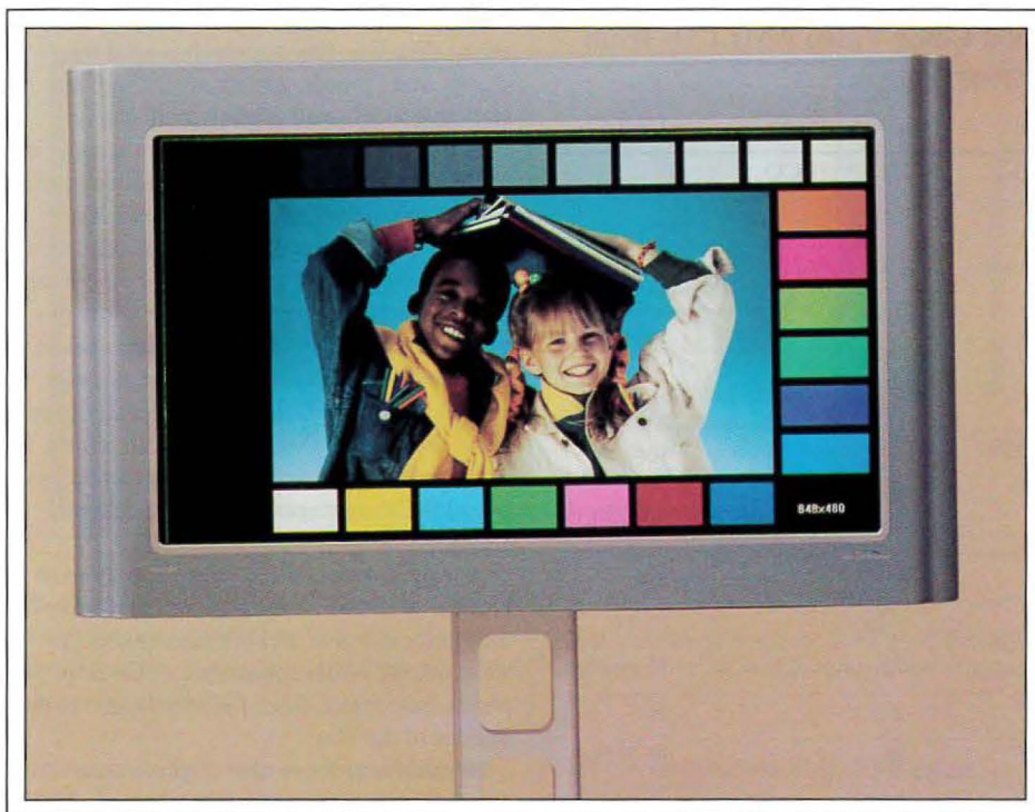
Fig. 2: Rainbow Display's 37.5-in. WVGA SDTV display is composed of one row of three tiled AMLCDs, with vertical seams. (The image on the display is from the 1999 ICIA INFOCOMM Shoot-Out CD.)
