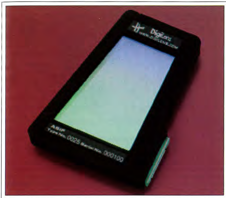
Fig. 2: This demonstrator was created by removing the color wheel from an InFocus 435Z front projector and replacing the fold mirror with a custom-fabricated ASIF.
