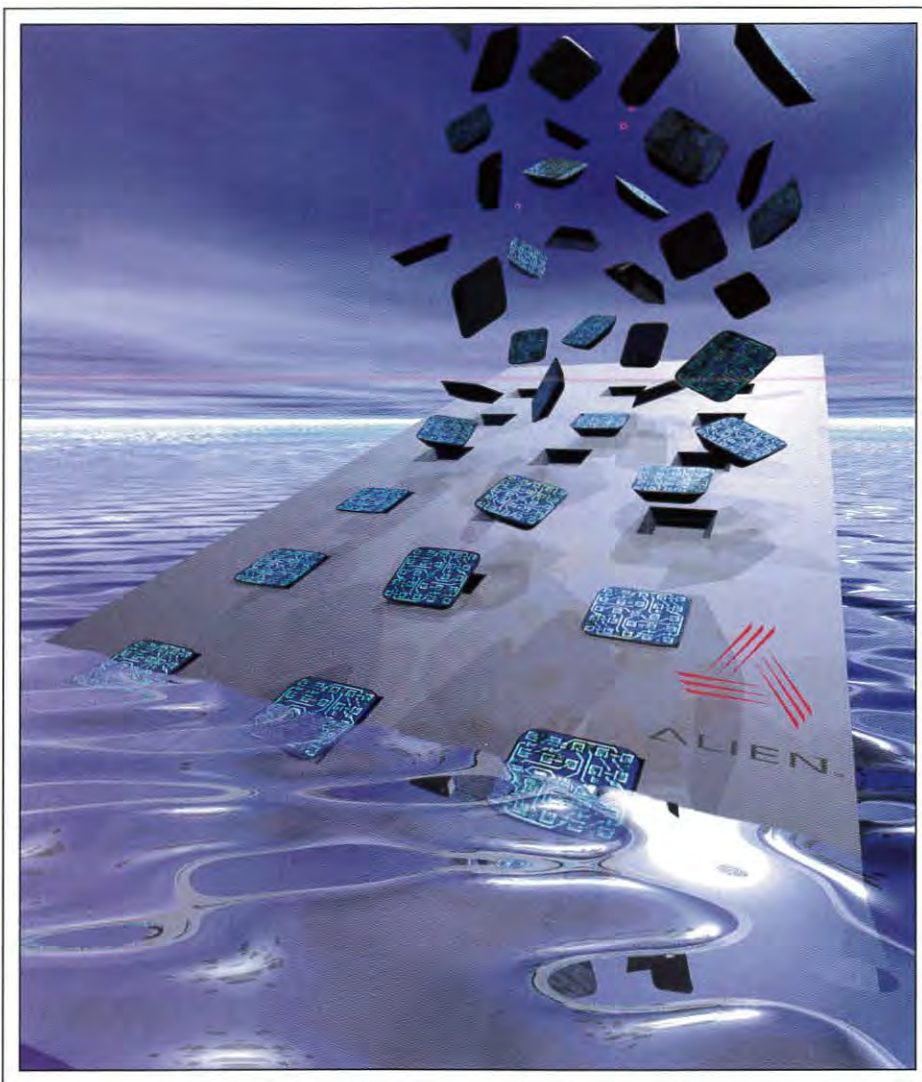
Fig. 1: This artist's rendering of the Fluidic Self-Assembly (FSA) process shows NanoBlock™ ICs falling into formed holes embossed in a substrate.
