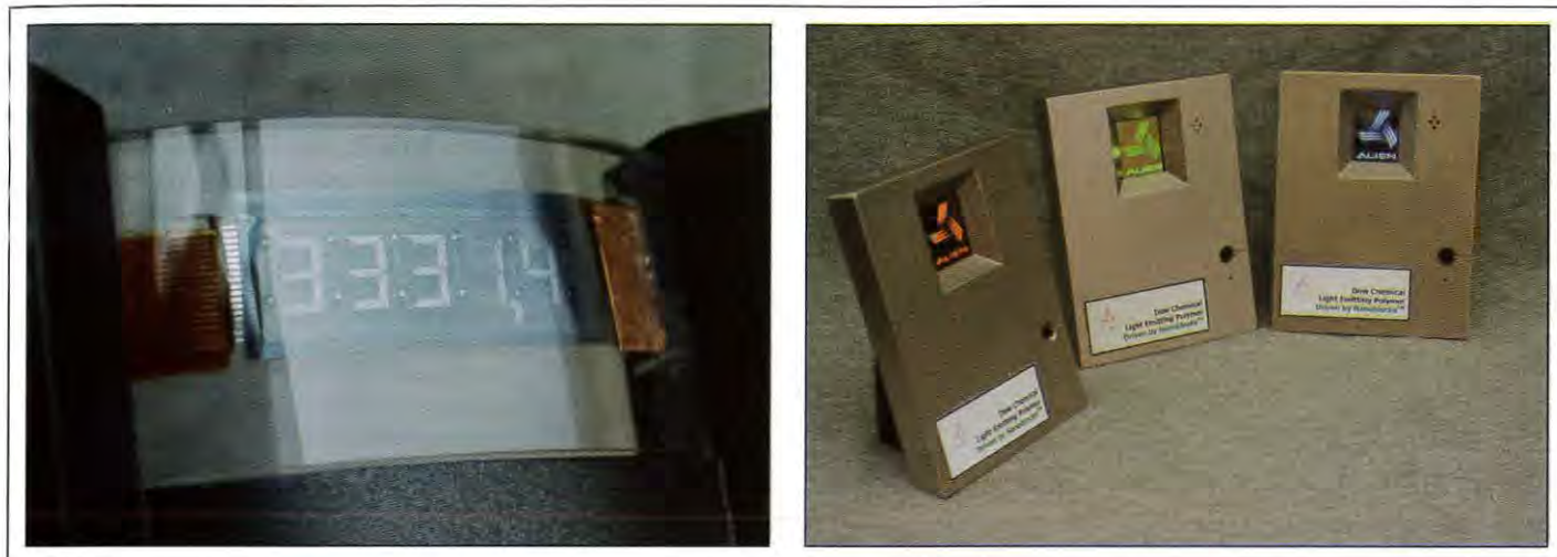
Fig. 7: A display in smart-card format, made with NanoBlock ICs placed by FSA into flexible plastic film, interconnected with deposited aluminum, and driving a 20-V PDLC film laminated onto the backplane is shown at the left. Red, green, and blue polymer-LED displays made from Dow Chemical material and driven by NanoBlock chips are shown at the right.
