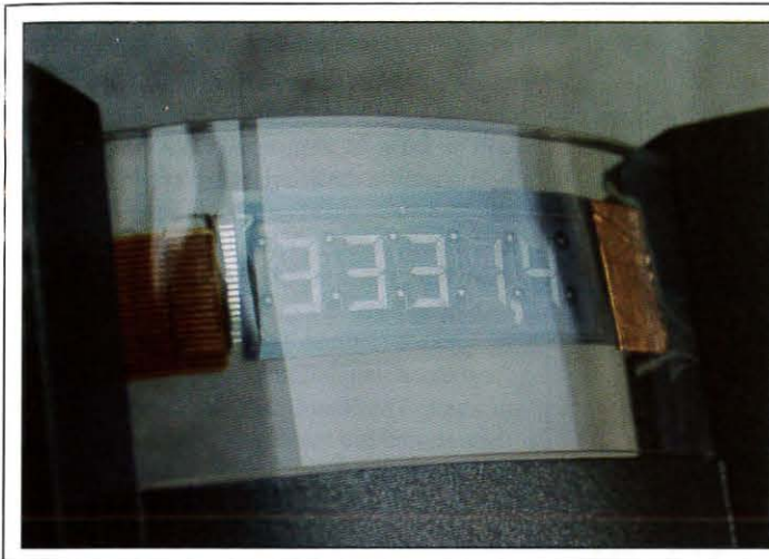
Fig. 7: A display in smart-card format, made with NanoBlock ICs placed by FSA into flexible plastic film, interconnected with deposited aluminum, and driving a 20-V PDLC film laminated onto the backplane is shown at the left. Red, green, and blue polymer-LED displays made from Dow Chemical material and driven by NanoBlock chips are shown at the right.
