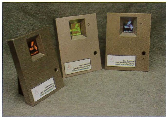
Fig. 7: A display in smart-card format, made with NanoBlock ICs placed by FSA into flexible plastic film, interconnected with deposited aluminum, and driving a 20-V PDLC film laminated onto the backplane is shown at the left. Red, green, and blue polymer-LED displays made from Dow Chemical material and driven by NanoBlock chips are shown at the right.
