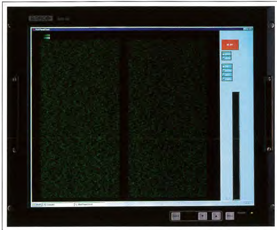
Fig. 3: When sonar operators first attempted to use 20-in. LCDs to view "waterfall-gram" data from sonobuoys, as pictured here, a disruptive blinking made it impossible for them to do their jobs.
