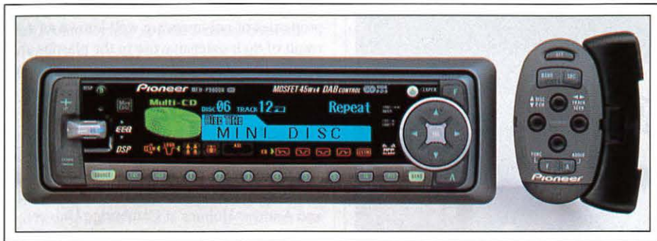
Fig. 2: Pioneer is currently producing multicolor organic electroluminescent displays for automotive audio products.
