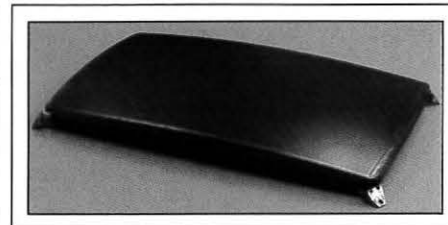
Fig. 4: A doubly curved mask - similar to those used in curved-faced CRTs - can be used in flat-faced designs.
