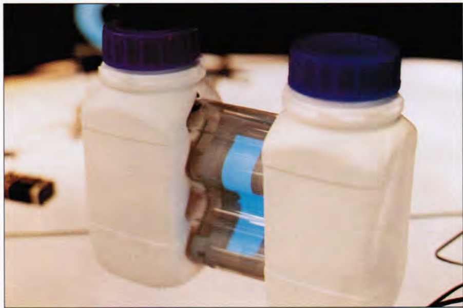
Agfa-Gevaert used the exhibition to show that its new Orgacon film with organic conductor (intended to replace ITO) is flexible. This curvaceous EL lamp was one of several demonstrators.
