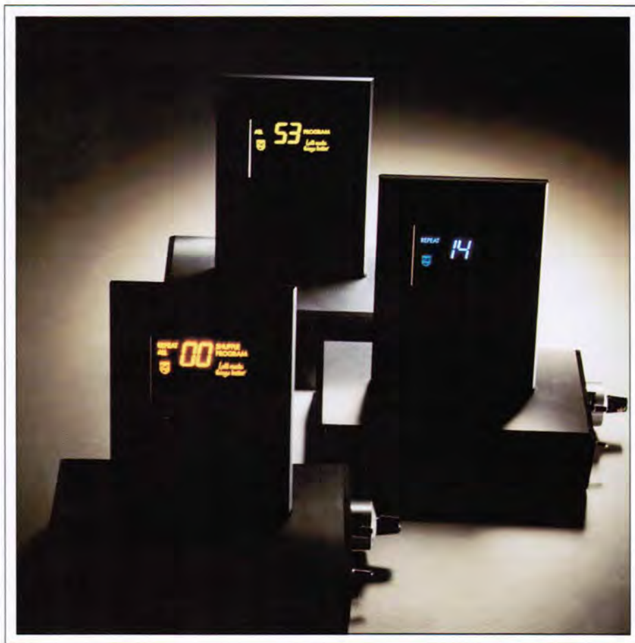
Fig. 2: Poly-LEDs have improved dramatically. All colors are now available, efficiencies are extremely high, and lifetimes – currently in excess of 10,000 hours for some colors – have improved by factors of 10 each year.
