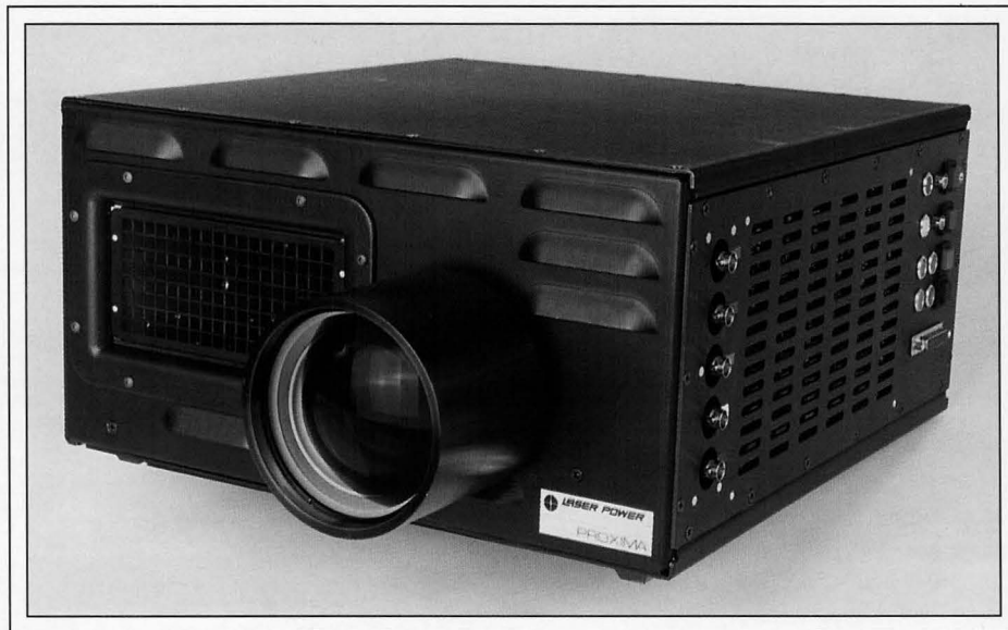
Fig. 4: A prototype air-cooled laser-illuminated portable LCD projector is fully self-contained and has dimensions of 15 × 15.5 × 8.5 in.
