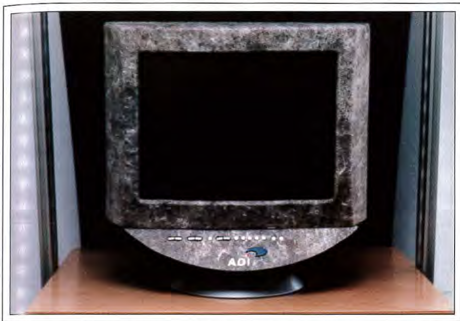
Fig. 4: ADI showed a monitor cabinet that is really green – although it may appear more like brown in this photo. Half flax and half cellulose diacetate, the composite material of which the cabinet is made can be put in a compost pile and returned to the soil – presumably after the monitor stops functioning.
