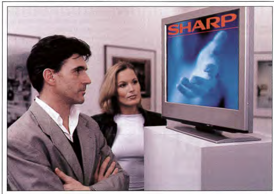
Fig. 3: Sharp attracted attention at CeBIT with a prototype 28-in. TFT-LCD video monitor, the LC-28HM2, featuring a resolution of 1280 × 768.
