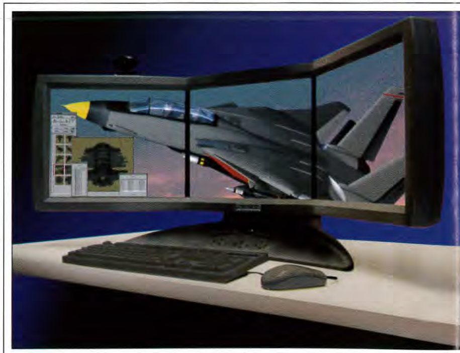
Fig. 1: Among the more interesting displays at National Manufacturing Week was a very-wide-format AMLCD from Panoram Technologies consisting of three SXGA panels with small millimeters between them.
