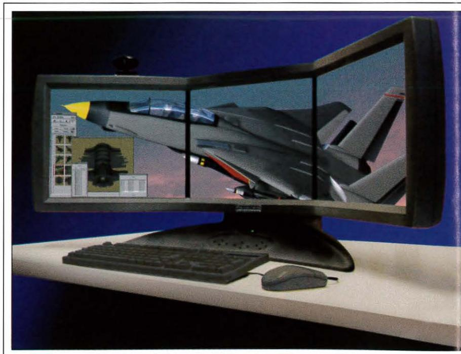
**Fig. 1:** Among the more interesting displays at National Manufacturing Week was a very-wide-format AMLCD from Panoram Technologies consisting of three SXGA panels with small multi-lions between them.
