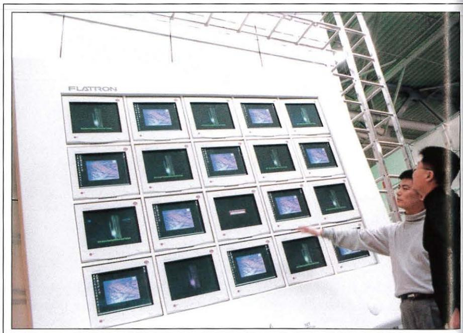
**Fig. 1:** "Perfectly," "naturally," and "purely" flat CRT monitors were an important – even dominant – part of many CRT lines at CeBIT 2000. LG Electronics was uninhibited in showing off its Flatron™ line, which is unusual in that the inner surface of the tube's faceplate, as well as the outer surface, is flat.
