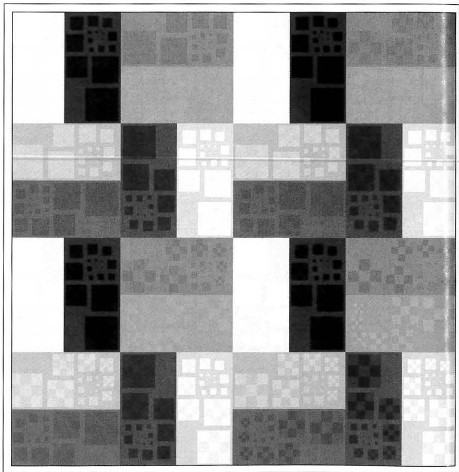
**Fig. 1:** The Briggs Test Pattern is a sequence of checkered patterns that takes into account the eye's ability to resolve features of decreasing size at different luminance levels with varying background luminance levels. The pattern provides an intuitive way of assessing the display's contrast modulation. (Source: Stewart Briggs, SPIE Vol. 762, "Electro-Optical Imaging Systems Integration," 1987.)
