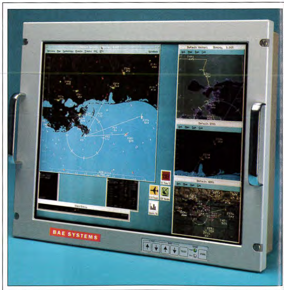
Fig. 1: BAE SYSTEMS has integrated NEC Technologies' commercial AMLCD into a rugged 20-in. flat-panel monitor for military applications.
