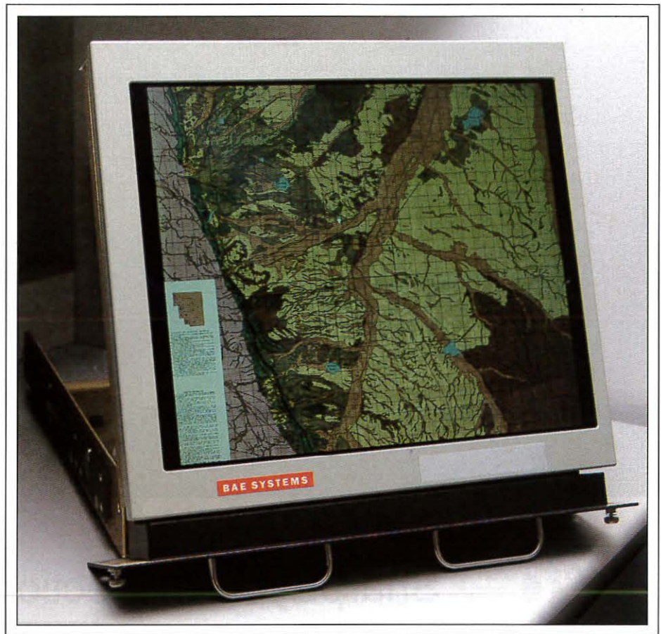
Fig. 4: The flexibility of an open-architecture modular design permitted the 20-in. monitor to be adapted for installation in a drawer for a 19-in. rack.
