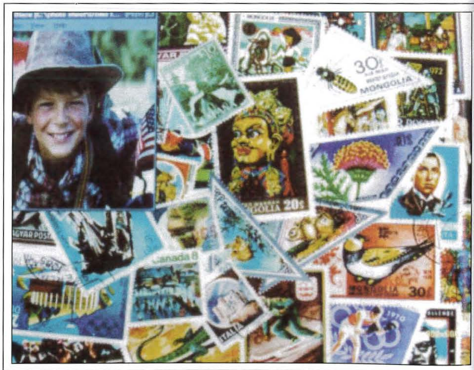
Fig. 1: FED picture content is increasing. This 13.2-in.-diagonal ThinCRT™ has 800 × 600 pixels with a 200-cd/m 2 luminance and 200:1 contrast ratio.
