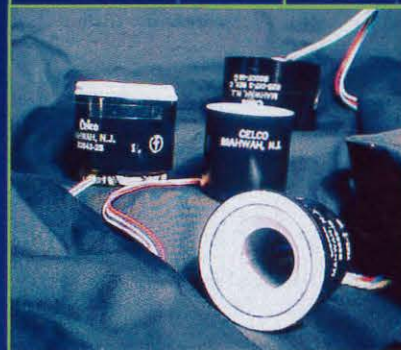
Left: Commercial Head-Up Display Yoke Top: Flight Mgt. Display Yoke Bottom: F-18 Map Display Yoke
