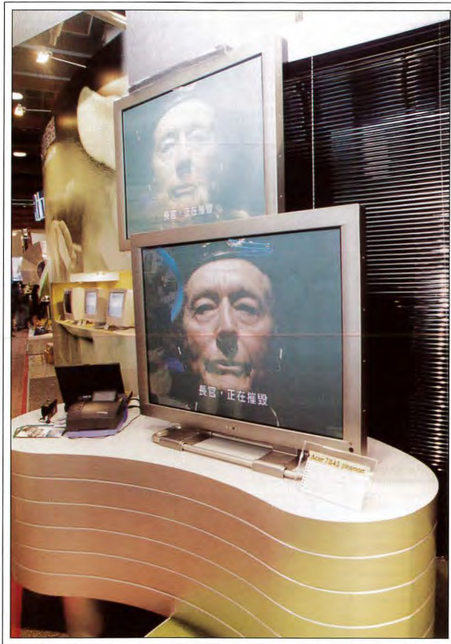
Fig. 4: Acer attracted attention at Computex Taipei with its new 42-in. PDP, the "very first Taiwanese-made color plasma-display panel." First shown in prototype form at the Asia SID (ASID) conference in March, the panel has an aspect ratio of 4:3, 350-nit luminance, and SVGA screen.
